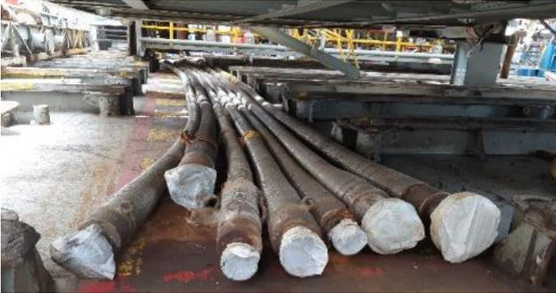
The lengths of flexible Choke and Kill lines stored under the drilling packages on the pipe deck.
