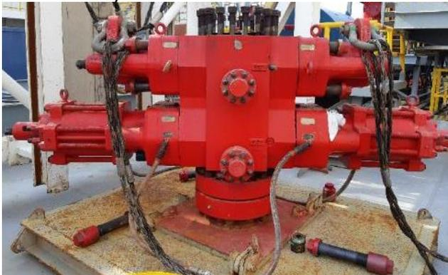
The 13-5/8" double BOP mounted on its test stump.
