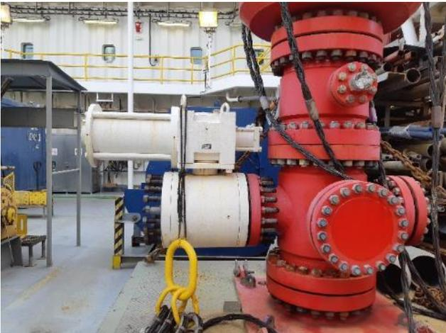
The diverter flow spools under the Diverter 21-1/4" Annular, showing the 1 x 12" overboard discharge ball valve installed on the bottom flow spool.
