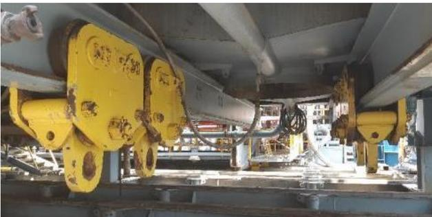
The 4 x I-beam trolleys that are used to hang the BOP hoist off. No SWL is visibly displayed on these I-beam hoists.
