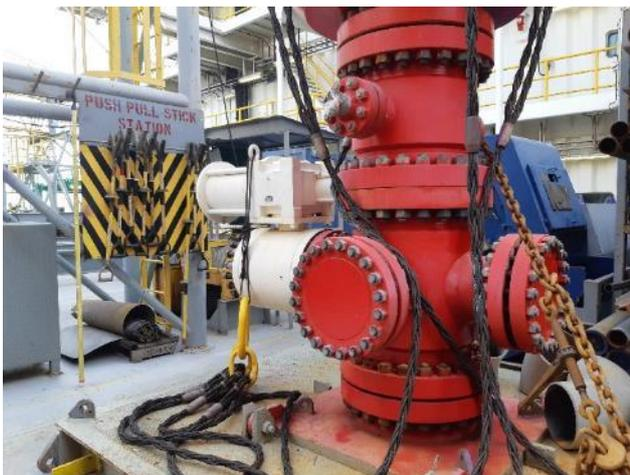
The diverter flow line spools mounted on to the test stump used for the 21-1/4" Annular and ram BOP's.
