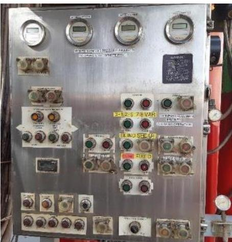
The Drillers BOP / Diverter remote control panel on one of the drilling the packages mounted between the MGS and Choke and Kill manifold.
