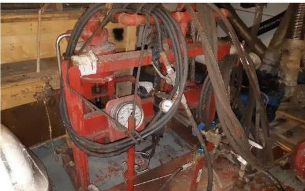
The BOP test pump assembly stored in the sack store.
