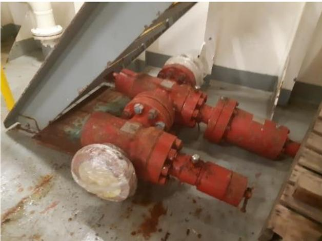
The Kill line valves associated with the Low-Pressure BOP's, were stored in the rigs sack store. No documentation was issued or sighted by the MS surveyor to relation to these valves
