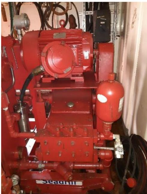
The electric driven hydraulic pump installed on the BOP / Diverter accumulator unit.
