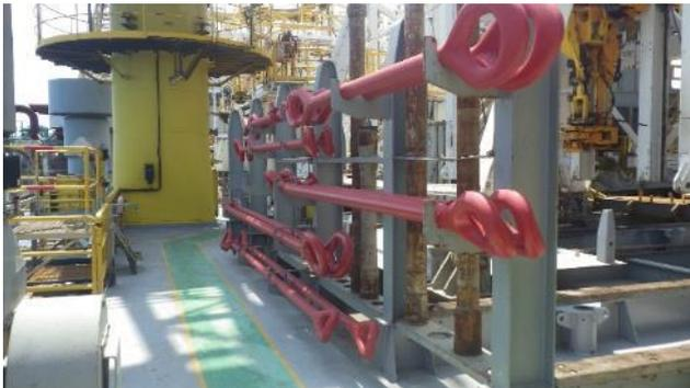
The links were in storage during the inspection and were found to be corrosion free and well stored.
