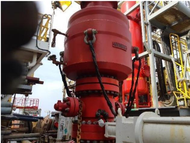
The Diverter assembly with the 21-1/4" Hydril MSP annular installed on top of the diverter flow line spool piece.
