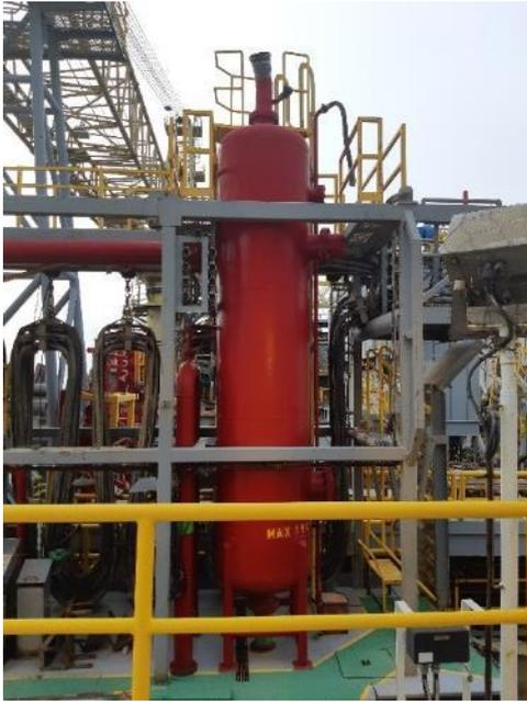
Mud-Gas Separator with minimum 30" OD vessel, minimum mud seal of 12 feet and one of the outlets connected to 8" OD gas vent line.
