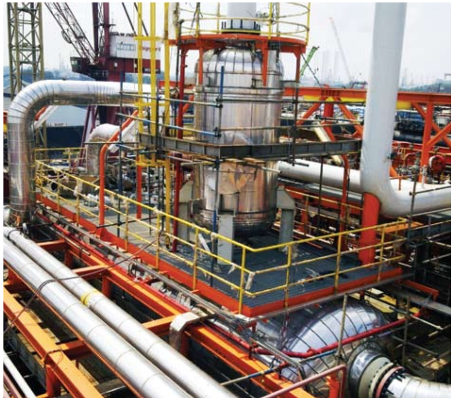
■ Sep-iSYS™: Separator with Integrated Polishing Scrubber for Floating Production Storage and Offloading (FPSO) vessel in Vietnam
