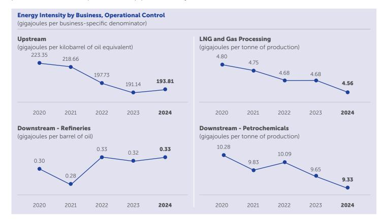
There is a general downward trend in energy intensity between 2020 and 2024, showcasing improvement in energy efficiency. The increase in energy intensity in refineries, including a sudden spike from 2021 to 2022, due to the upgrade of the Melaka refinery to meet EURO V Diesel product specifications, in compliance with the Environmental Quality (Control of Petrol and Diesel Content)
