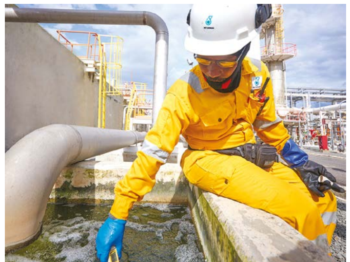
A PCG technician takes wastewater sample for analysis of COD, as an indication of how much organic matter is released into surrounding waters
