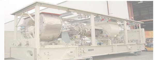
Additional compressors at Segamat Compressor Station
