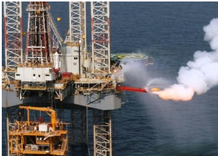
Figure 4-10: Flaring in an Exploration Drilling Campaign
