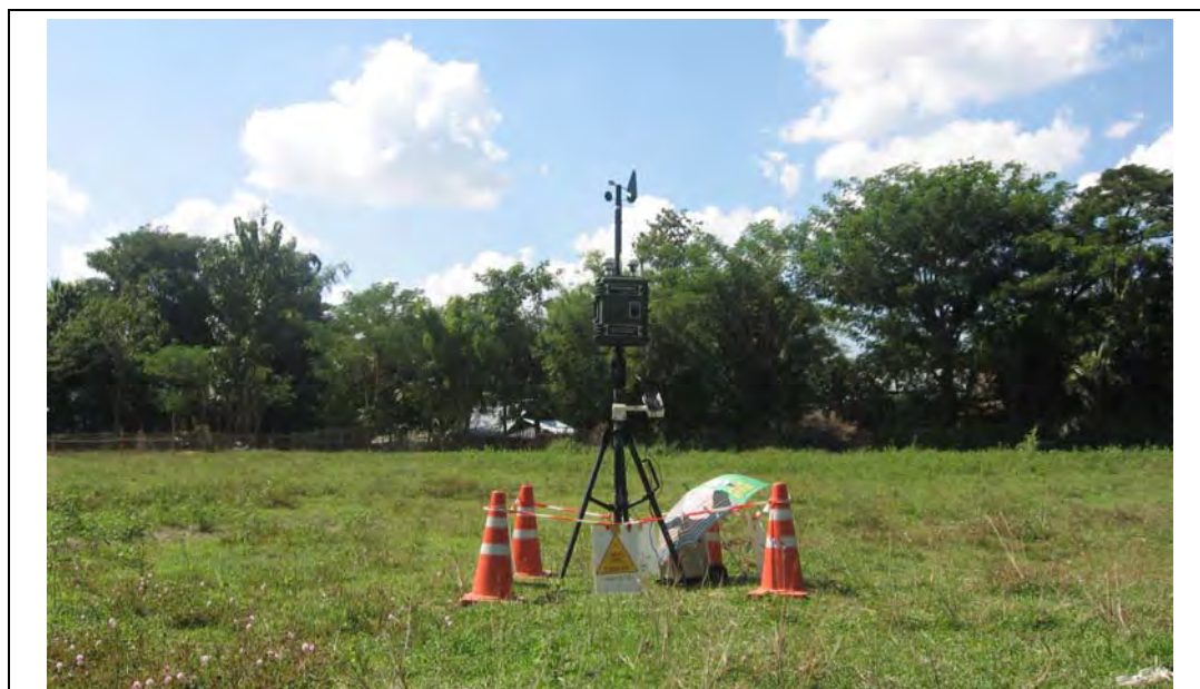
Plate 3-5: Ambient air monitoring station in Zee Kone village
